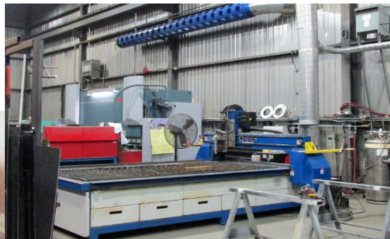
INDOOR PLASMA MANUFACTURING AREA CONNECTED TO AN OUTDOOR H8 CARTRIDGE DUST COLLECTOR
