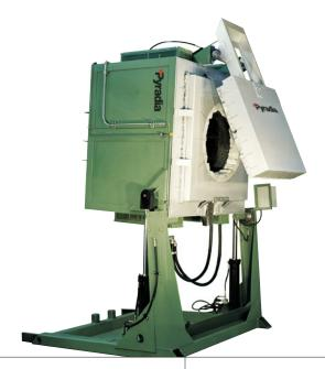
This furnace has a capacity of 2,000 lbs. Isolated with ceramic fiber, it is equipped with silicon carbide heating elements and an optional hydraulic activated cover. See the last page for more information on the FCBC 320 model.
