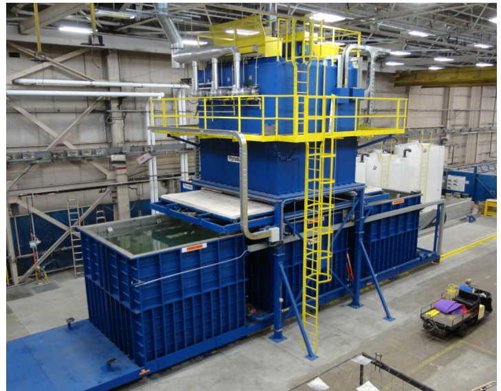
State of the art indirect gas fired Drop Bottom Furnace is class II
