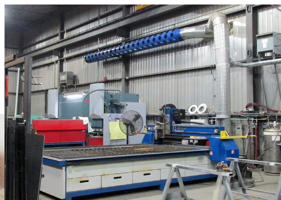
INDOOR PLASMA MANUFACTURING AREA CONNECTED TO AN OUTDOOR H8 CARTRIDGE DUST COLLECTOR
