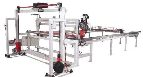
Light roll-floor pickup unwind stand with integral sheeting station.
