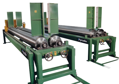
Driven surface unwinds with side paddle roll containment.
