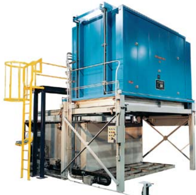
The sliding door oven shown is of standard configuration and was custombuilt to accommodate 7-feet/213 cm long parts. It is equipped with an optional motorized cart and the operator console is mounted on the oven. The quench tank is insulated and is equipped with a recirculation pump, immersion heater and chiller.
