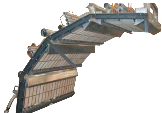
Electrical or gas fired IR dryers can be used as a complete IR unit or a combination convection-IR dryer. This has 16 control zones in machine and cross-machine directions.
