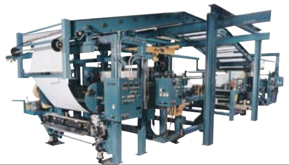
This water base PSA coating line operates up to 1200 FPM and is equipped with fully automatic turrets (dryers not shown).
