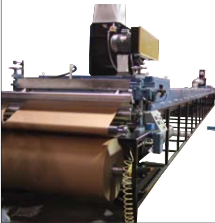
This gravure & knife combination coater is designed to operate up to 800 FPM. It features a pull roll assembly, an offset pivot guider and micrometer adjustments on the enclosed coating chamber and knife assembly.
